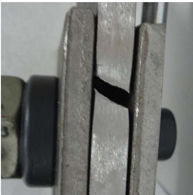
Photograph 5. Fracture of base material (M2)
