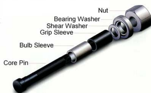
Figure 1 Components of High Strength One-Side Bolt
